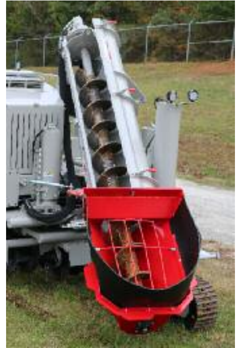
Auger Conveyor; lid opens for cleaning.
