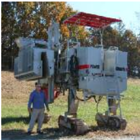
5700-D-MAX equipped with barrier mold lift.
