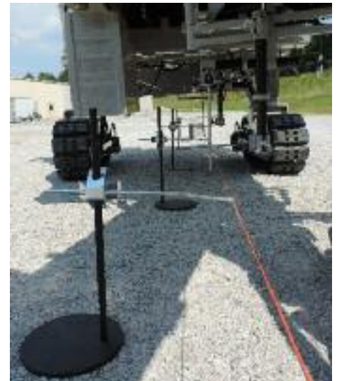
Parapet sensor mounting.
