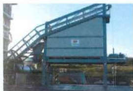
210 tonne load-cell mounted
