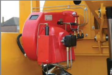
Batch heater light diesel oil burner
