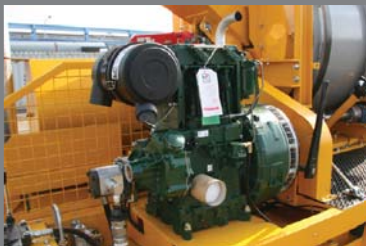
Diesel engine power drive
