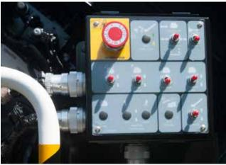
Ground level control boxes also feature improved layout and are backlit as well.
