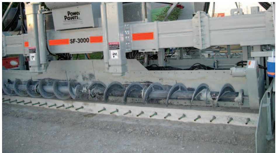
The sideforms widen allowing the machine to begin paving off an existing header. Hand tie-in work is minimized resulting in a better quality and smoother pavement.
