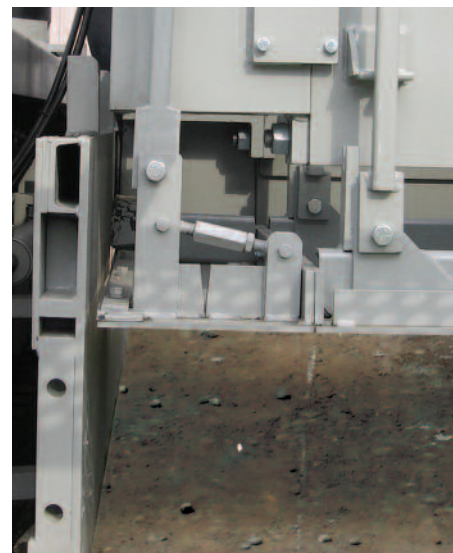
Edge overbuild feature compensates for edge slump
